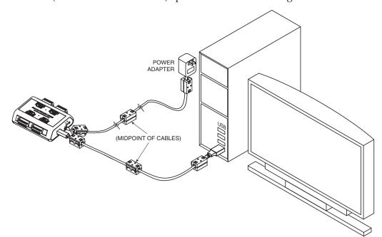
Figure 6-1. OM-DAQ-USB-2401 with Ferrite Cores Installed
